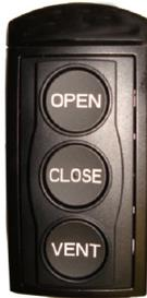
To **Close** the glass panel from any position, press once (one-touch function). For manual function, hold the close button.
